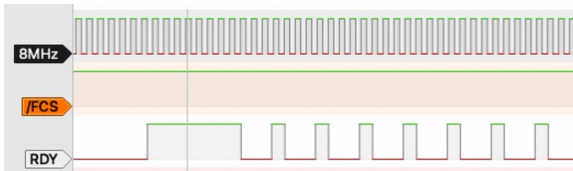
Picture 1: DMA data transfer - /FCS remains at HIGH level
