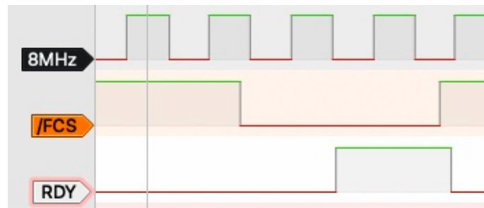
Picture 2: DMA register access – C025913-38 without modification of the signal RDY
