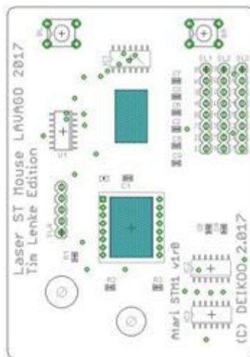
The board has three ports that fits most original Atari mouse cables.
