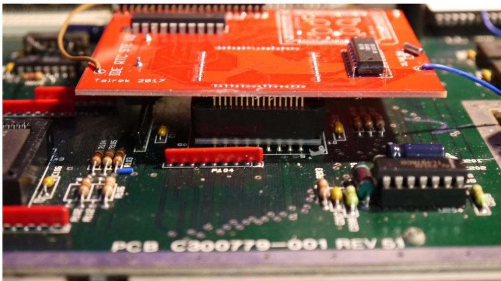
3.4 Prepare the interface by plugging in the wire to the pin no 10 of the ACSI port.
